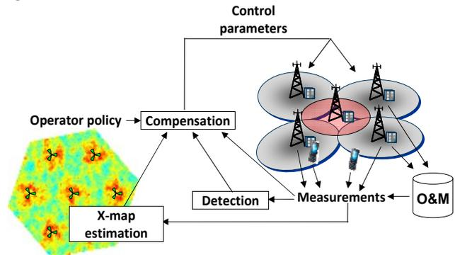
Figure 3: Cell outage management components. The center site is in outage. Red area indicates the coverage previously offered by the outage cell (Source: [5])
